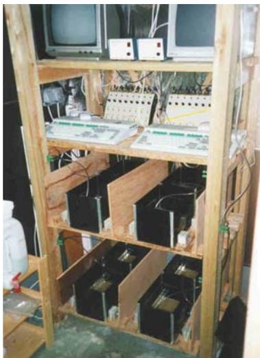
Figure 3- Actograph system showing tanks, infrared emitters/detectors and control computers.
