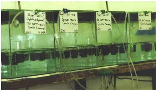
Figure 2- Moulting racks deployed in exposure tanks
