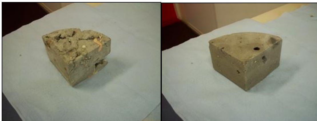
(a) APC residue + cement + metal sludge
