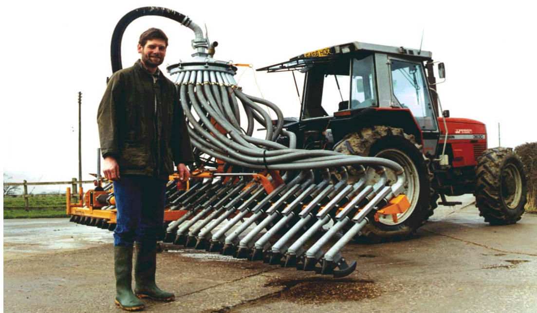
Figure 4. Veenhuis 6m trailing shoe boom at Berrowsfield Farm
