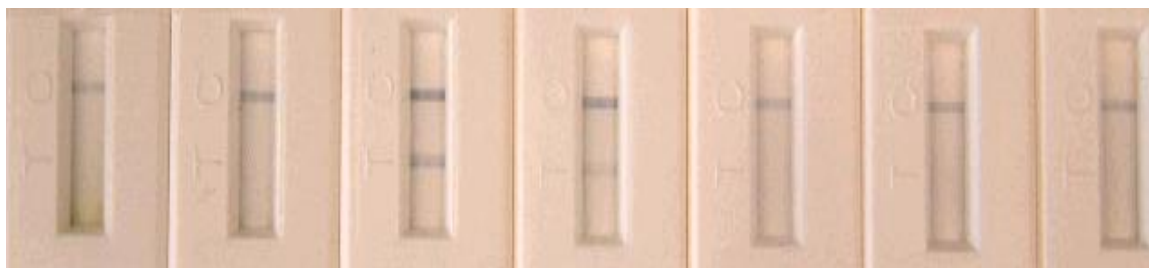
Figure 14: Photographs of prototype LFDs (1-7 left to right) following testing of a range of fungal and other plant pathogens. 1 = Healthy leaf (negative control), 2 = Generic Rhizoctonia sp. positive antigen (Neogen) at 5\mu\text{g ml}^{-1} , 3 = Generic Phytophthora sp. positive antigen (Neogen) at 5\mu\text{g ml}^{-1} , 4 = Generic Phytophthora sp. positive antigen (Neogen) at 0.5\mu\text{g ml}^{-1} , 5 = Erwinia amylovora bacterial suspension at 1 \times 10^7 \text{CFU} , 6 = Ralstonia solanacearum bacterial suspension at 1 \times 10^7 \text{CFU} , 7 = Buffer C (negative control)
