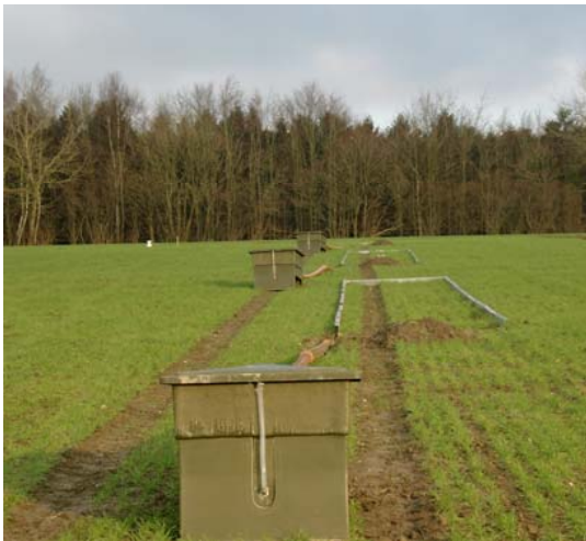
Figure 2. Experimental design at Pewsey showing (a) layout of replicate runoff traps, (b) capping of soil on traditionally cultivated treatment after heavy rain (Dec. 2002), (c) erosion on a late-drilled treatment before establishment, and (d) degree of crop cover on the reduced cultivated treatment (Dec. 2002).
