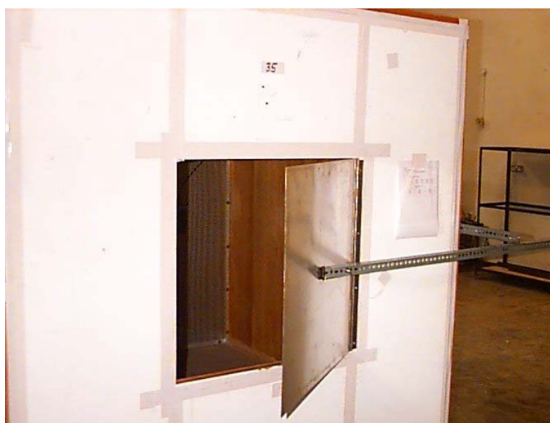
Fig. 1 A 0.7 m square vent and flap mounted on the end of the Fan Test Rig
