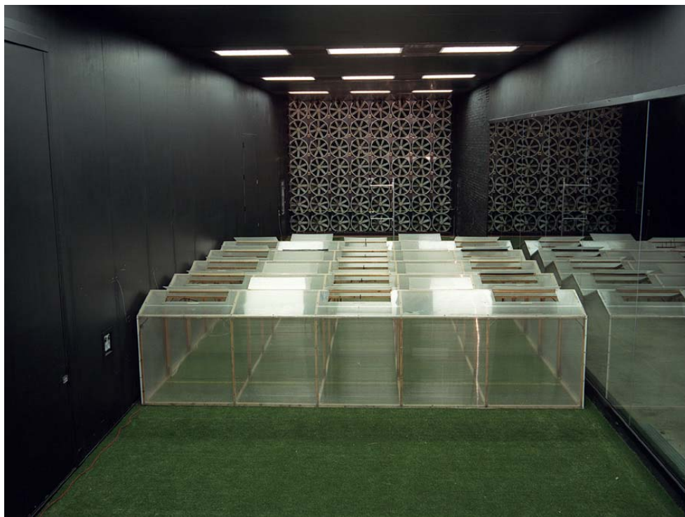
Fig. 3 View of model glasshouse looking upstream towards fans in AFL
