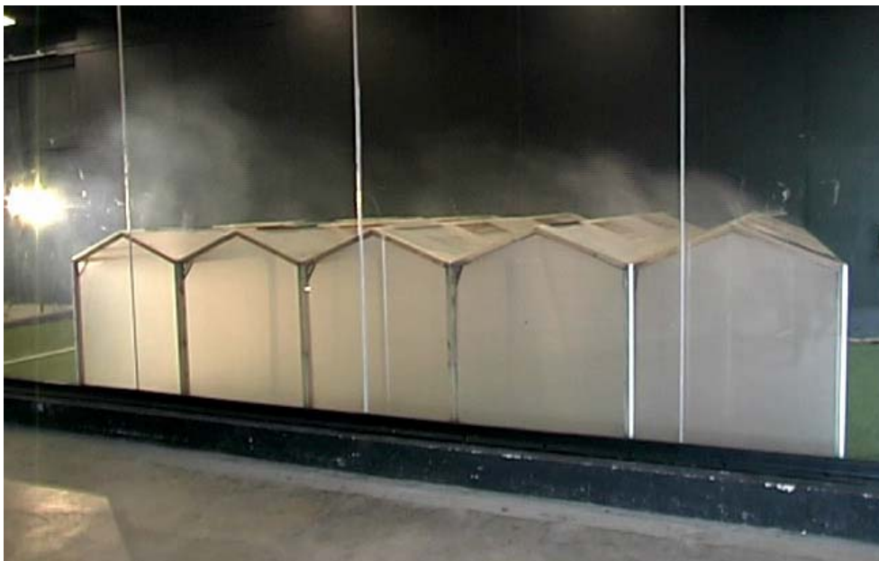
Fig. 12 Illustration of turbulent fluctuations producing outflow through downwind ventilators (top picture, left-hand end) and, a few seconds later, through upwind ventilators (bottom picture, right-hand end) for case when windward ventilators were 60% open
