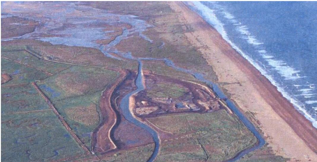
**Figure 1. Aerial photo during construction. This shows the old and new route of the River Glaven. The channel at the back (nearest the sea) is the old channel, with the new route on the left further inland. The wetlands are shown in the background. Photo courtesy of Environment Agency and National Trust**
