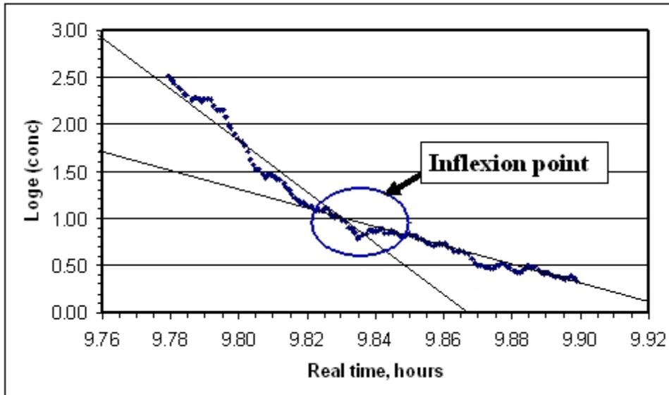
**Figure 7:** plot of  $\log_e C$  against time,  $t$  for first curve shown in Figure 6.
