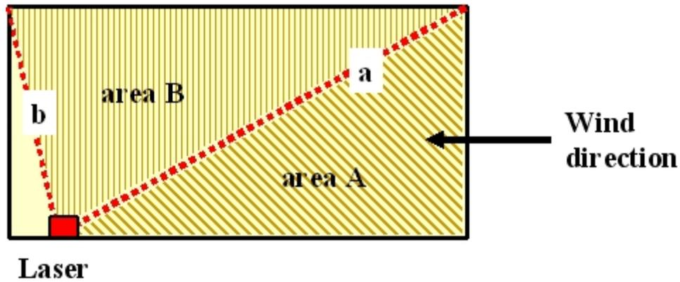
Figure 3: geometry of laser location with respect to the building being monitored.
