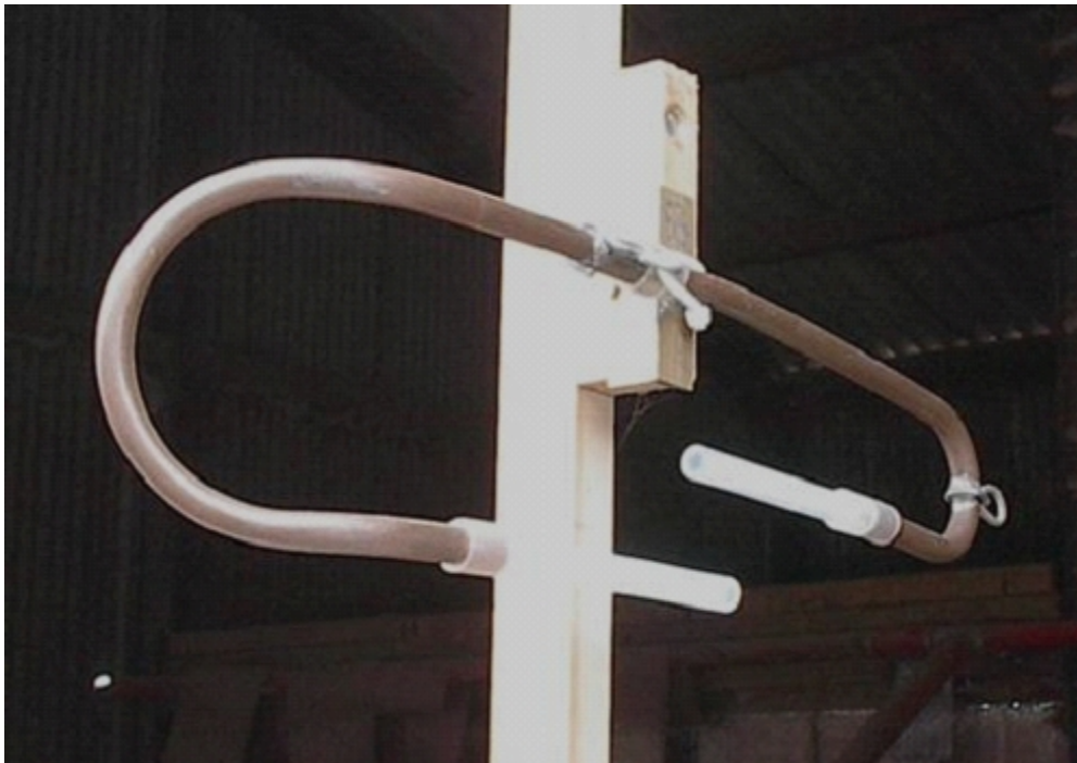
Figure 1: copper type of Ferm tube which represents the preferred design when deployment is possible. Example shown mounted in large opening on a suspended pole.
