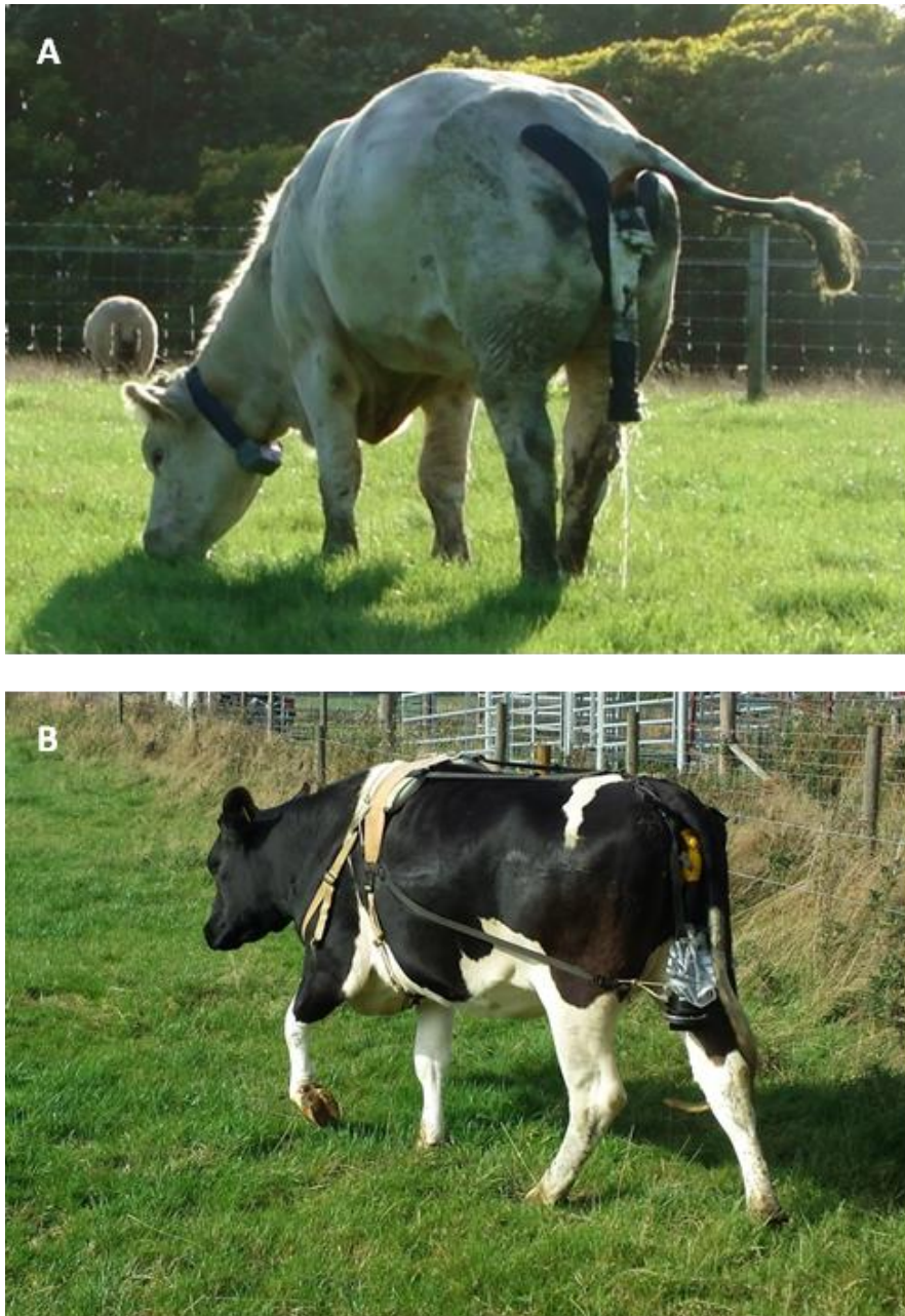
Figure 1. Attachment of urine sensor to the cow: A, showing initial configuration using Velcro straps glued to cow; B, final configuration using a harness with top and side straps to support sensor weight and minimise lateral movement. GPS collar also shown on the beef cow in A.
