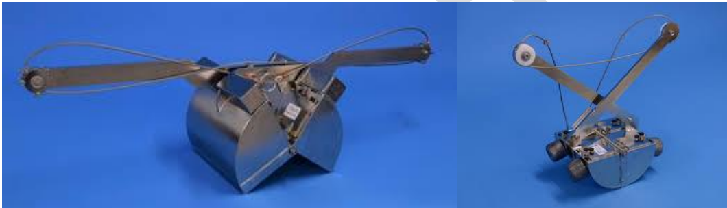
Figure A2 Van Veen grab sampler in armed and triggered positions (sourced from KC Denmark Research Equipment, 2016)
