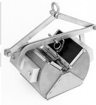
Figure A2 Van Veen grab sampler in armed and triggered positions (sourced from KC Denmark Research Equipment, 2016)
