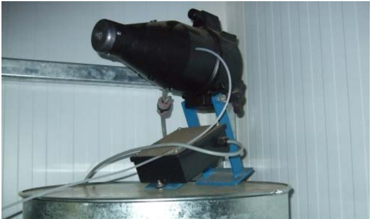
Figure 2. Cyclomatic cold fogging system used for application of caraway oil in large scale trial.
