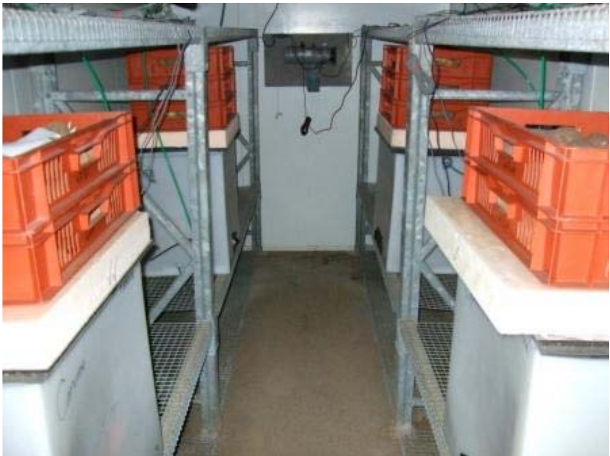
Figure 1. Experimental store showing four chambers for assessment of alternative sprout suppressants
