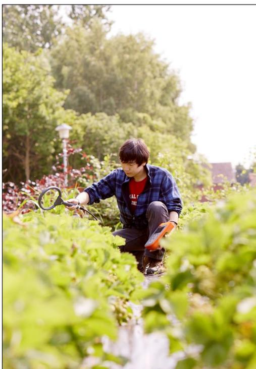
**Figure 5.** Detecting RFID tagged weevils within a commercial strawberry crop at Harper Adams University.
