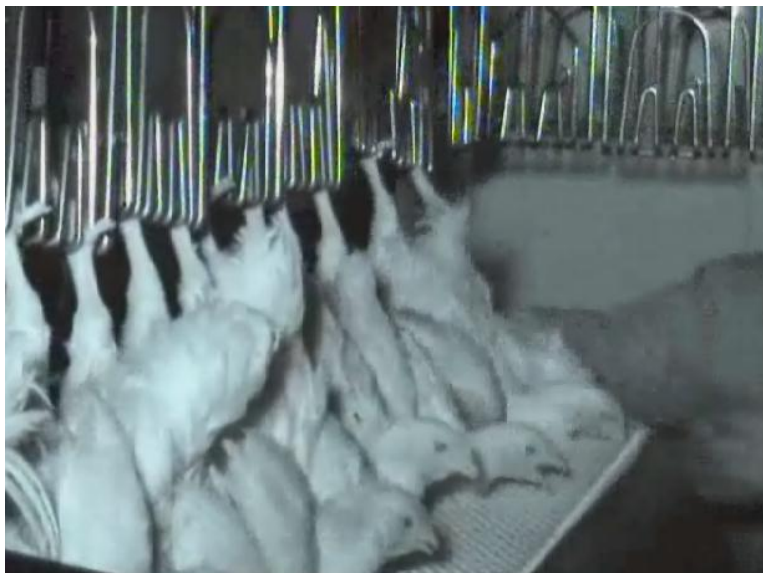
Figure 6 The hang-on section. The conveyor is too low in this photo, which results in some birds resting on their crops rather than on their breast
