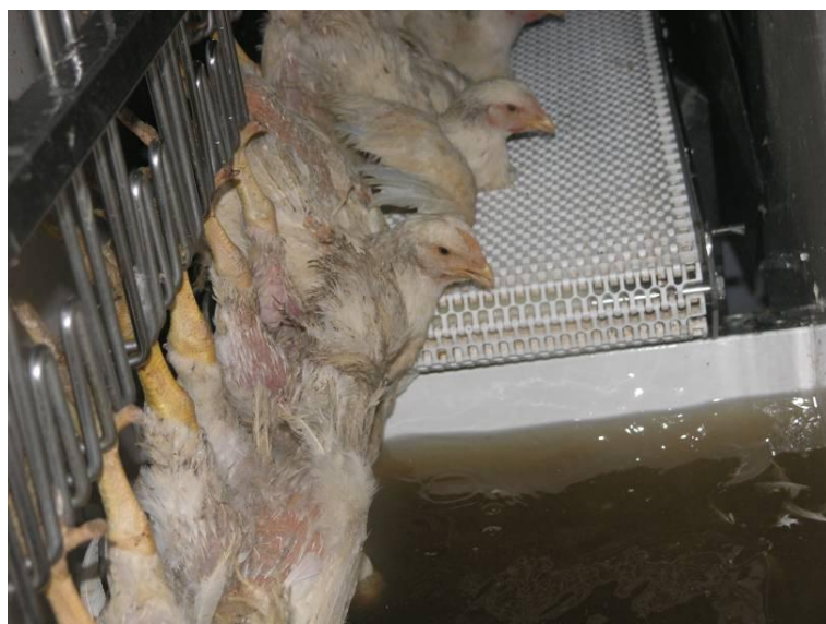
Figure 1 Birds passing from the conveyor into stun bath
