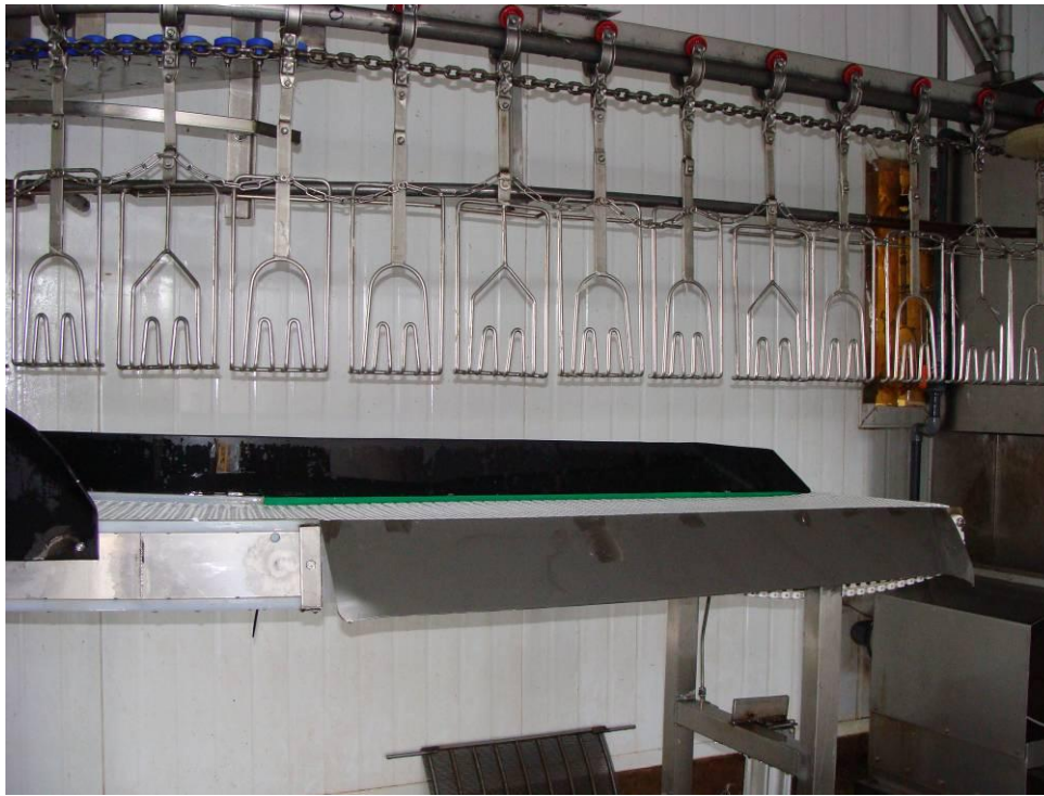
Figure 4 Breast support conveyor installed in processing plant
