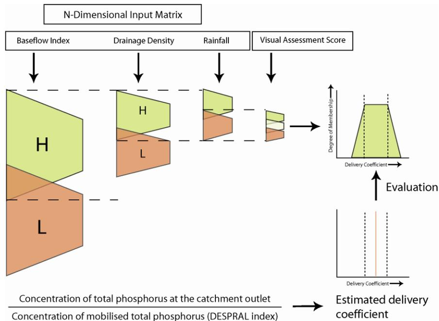
**Figure A2.3: Schematic diagram summarising the PEDAL approach and dual lines of approach used to evaluate the risk of P delivery. Modelled values for P delivery are obtained from a fuzzy decision tree approach using the BFI, drainage density and rainfall index to give coarse but nationally applicable fuzzy estimates of P delivery. The uncertainty of these derived estimates may be constrained by field measures of P delivery risk using the Visual Assessment**
