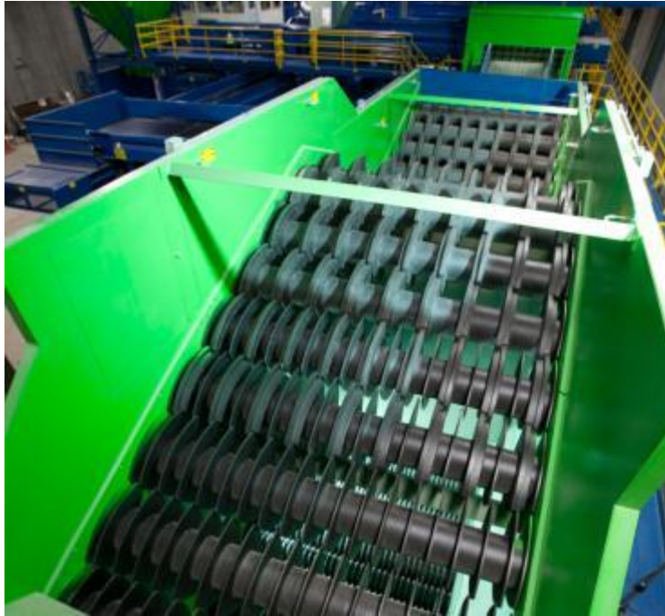
Figure 2 A disk screen separator showing the rows of rotating disks
