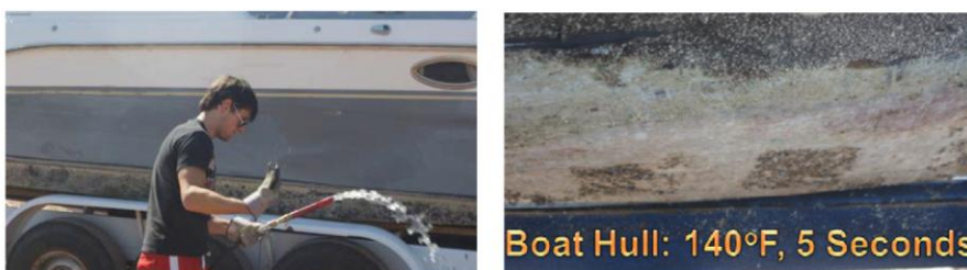
Figure 1. Images taken from a report produced by Wong showing boat cleaning using hot unpressurised water to effectively remove zebra mussels from boat hulls.
