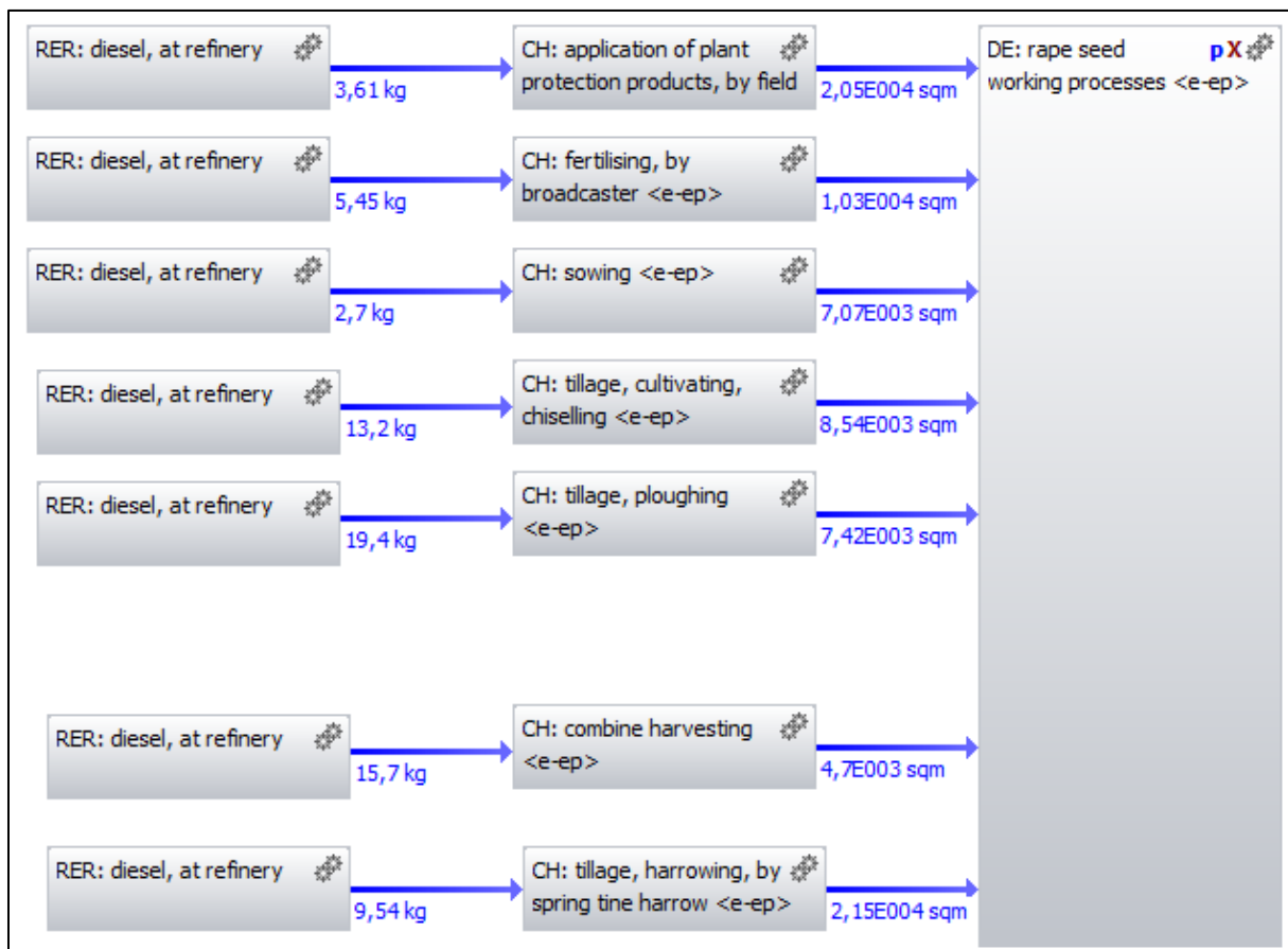
Fig. 5: Working processes for the production of rapeseeds scaled to the overall diesel consumption for rapeseeds production according to BIOGRACE Version 4c, which equals 69.6 kg diesel/ha
