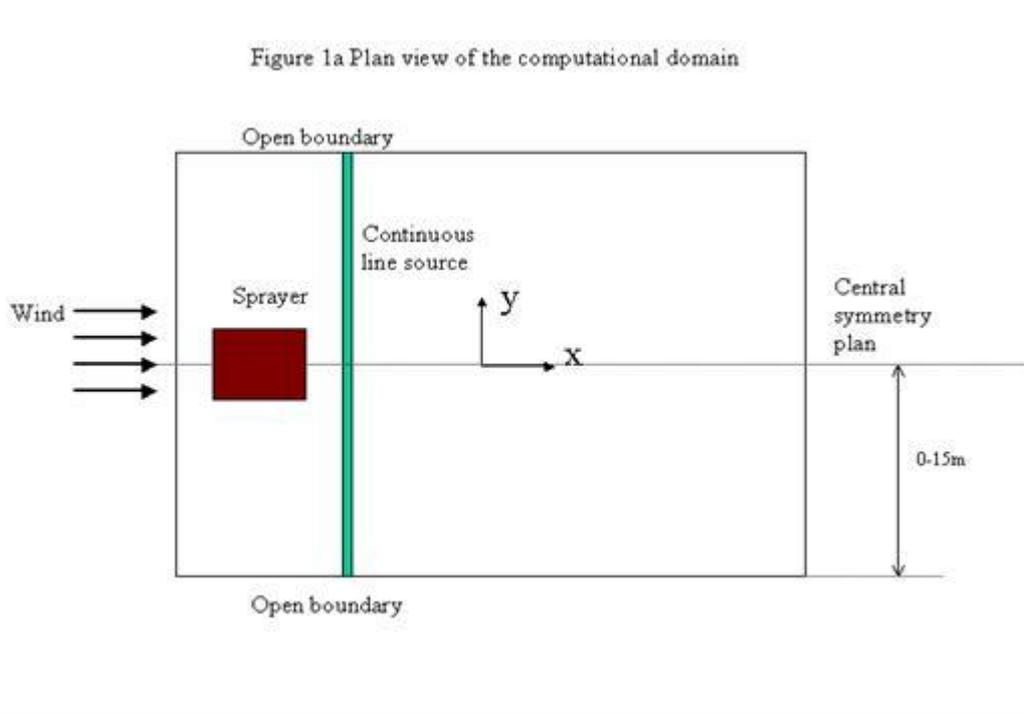
These results suggested that spray drift was unlikely to be increased by the presence of the sprayer, and that the drifting spray was potentially dispersed higher into the air by the airflows generated by the sprayer, and reducing airborne concentrations and potential human exposure
