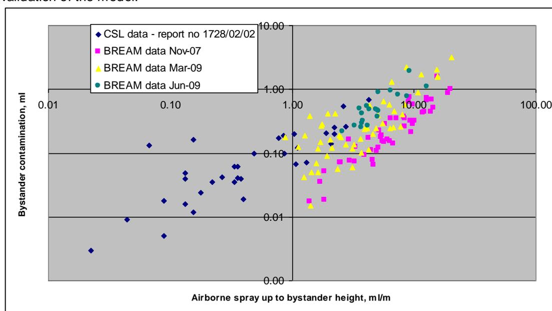
Figure 4. Relationship between mean airborne spray (ml/m<sup>2</sup>) x bystander height (m) and bystander contamination (ml)
