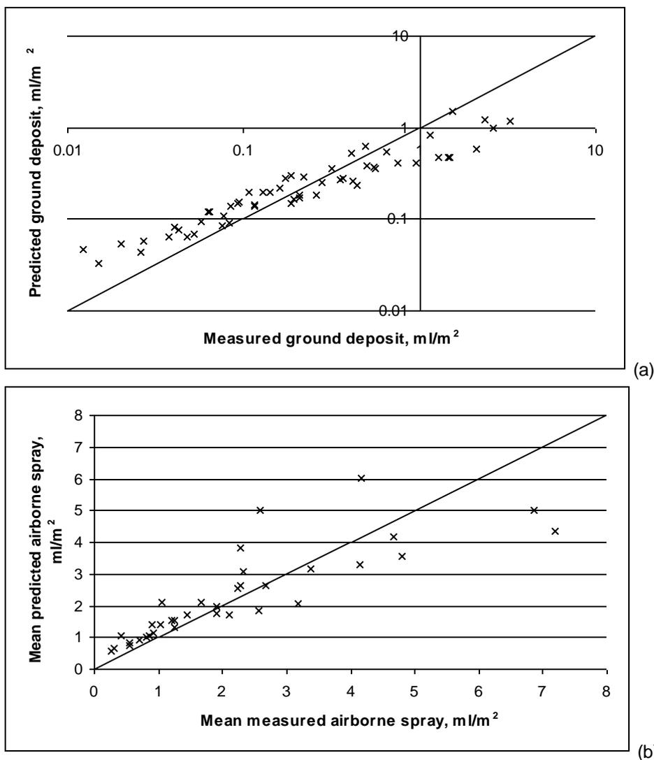
Figure 5. Comparison between measured and predicted spray drift between 2 and 20 m downwind for (a) ground deposits and (b) mean airborne spray from 0 – 2m above the ground. Flat fan nozzle (F/110/1.2/3.0) at 3.0 bar, 24 m boom, 12 and 16 km/h, boom height 0.7 – 1.1 m,
