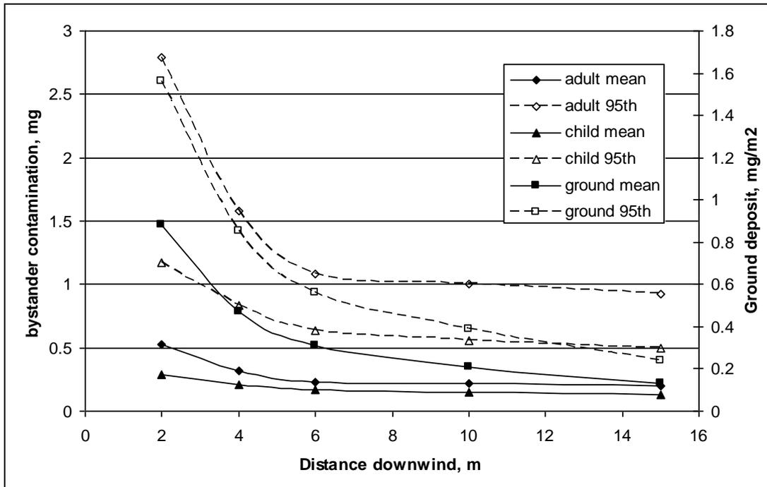
Fig 13. Model predictions of reduction in bystander dermal exposure and ground deposits with distance from the sprayer
