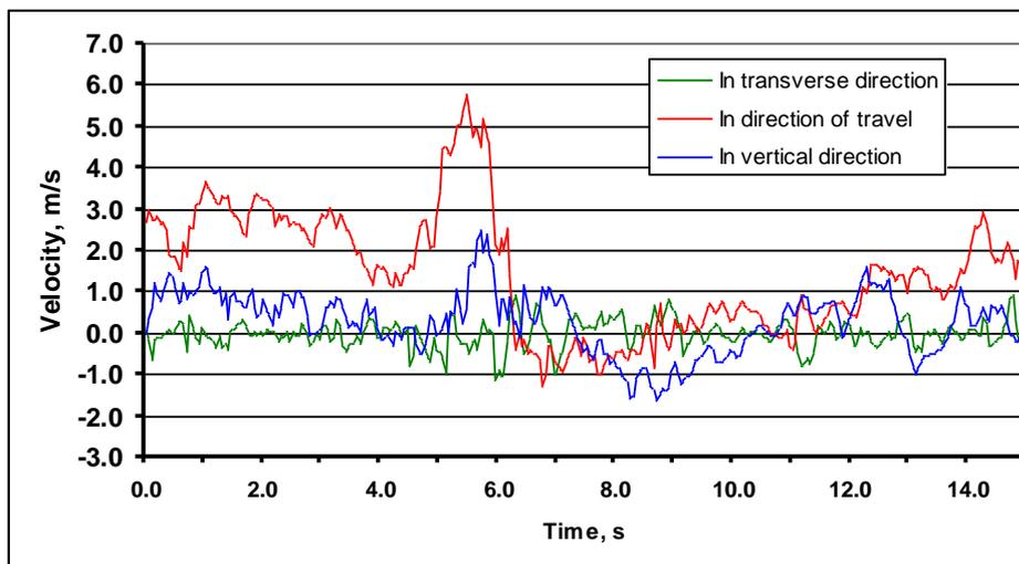
Figure 3. Time histories of air velocities measured as the sprayer passed over the anemometer
