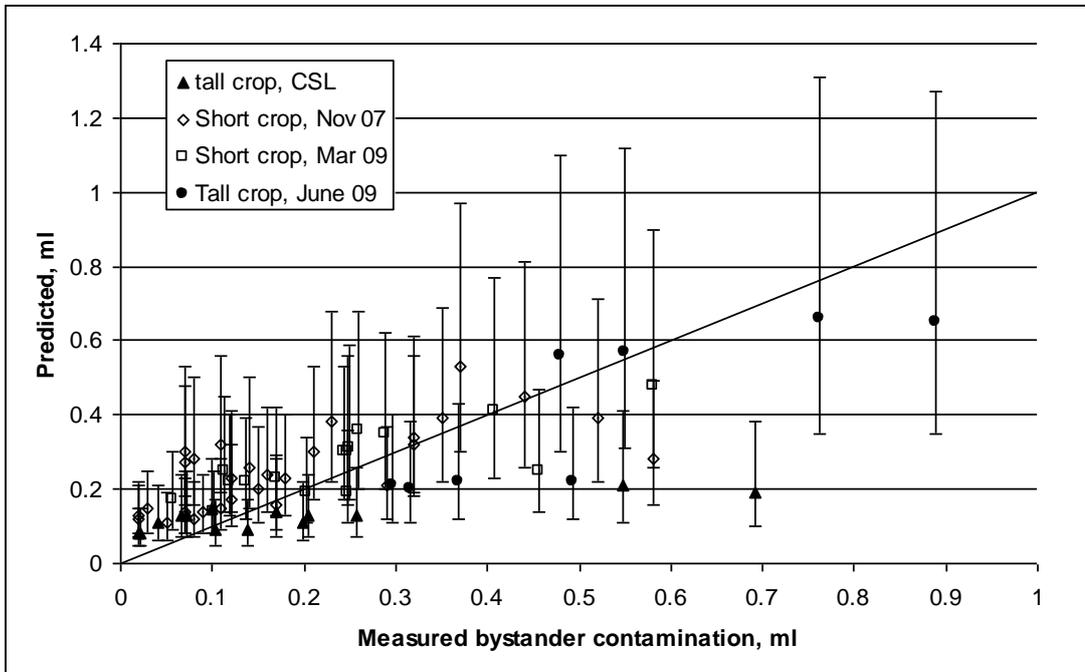
Figure 8. Comparison between measured bystander dermal contamination and that predicted by the BREAM model. Error bars refer to the 25th and 75th percentile predictions.
