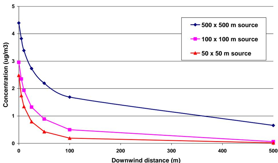
Figure 10 Decline of airborne concentration with distance downwind for different source (field) sizes.
