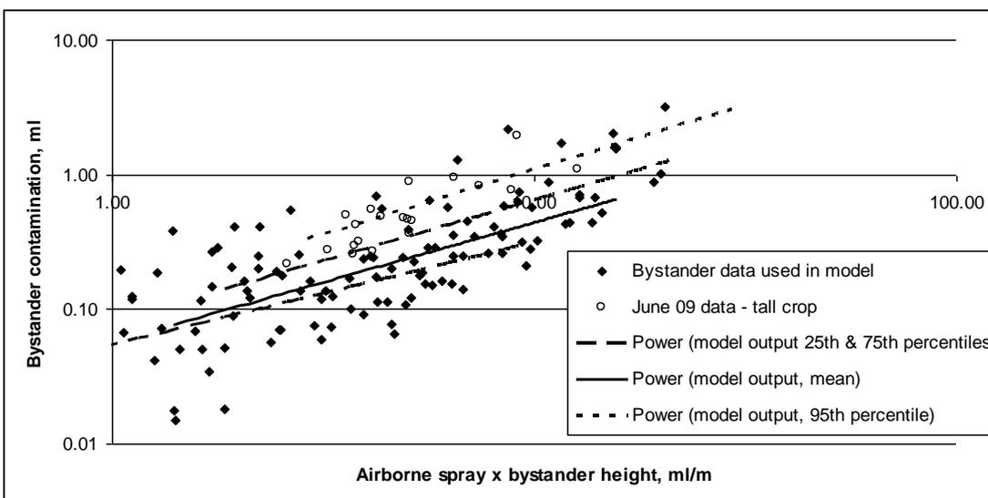
Figure 9. Relationship between airborne spray (ml/m<sup>2</sup>) x bystander height (m) and bystander contamination (ml) for experimental data and BREAM model output.
