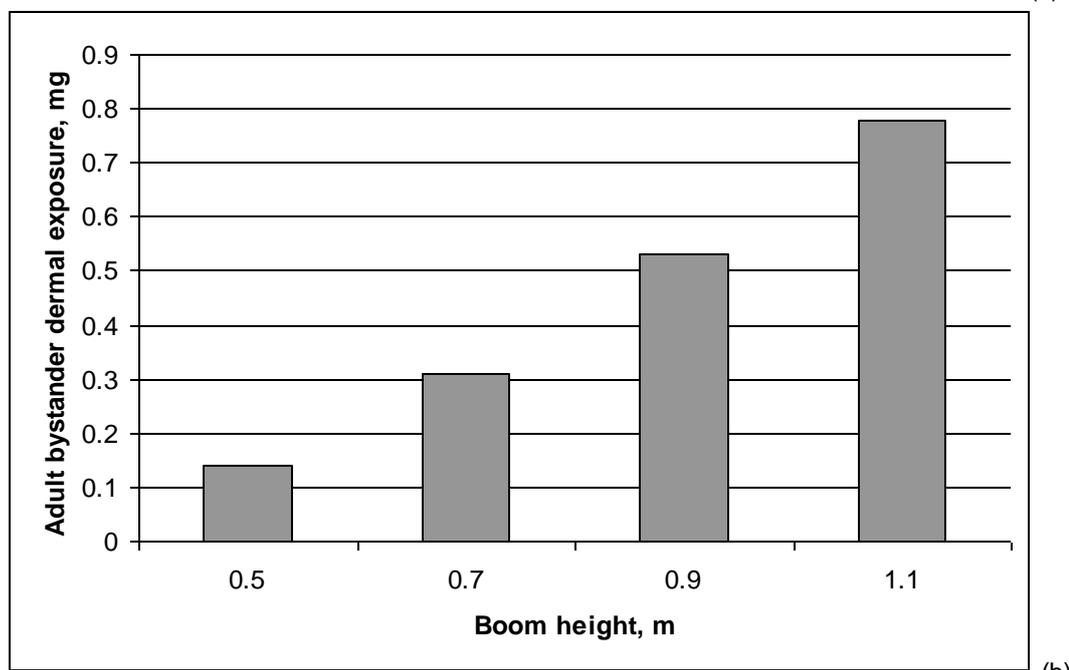
Fig. 11. The effect of (a) wind speed and (b) boom height on mean adult bystander dermal exposure, predicted at 2.0 m downwind.
