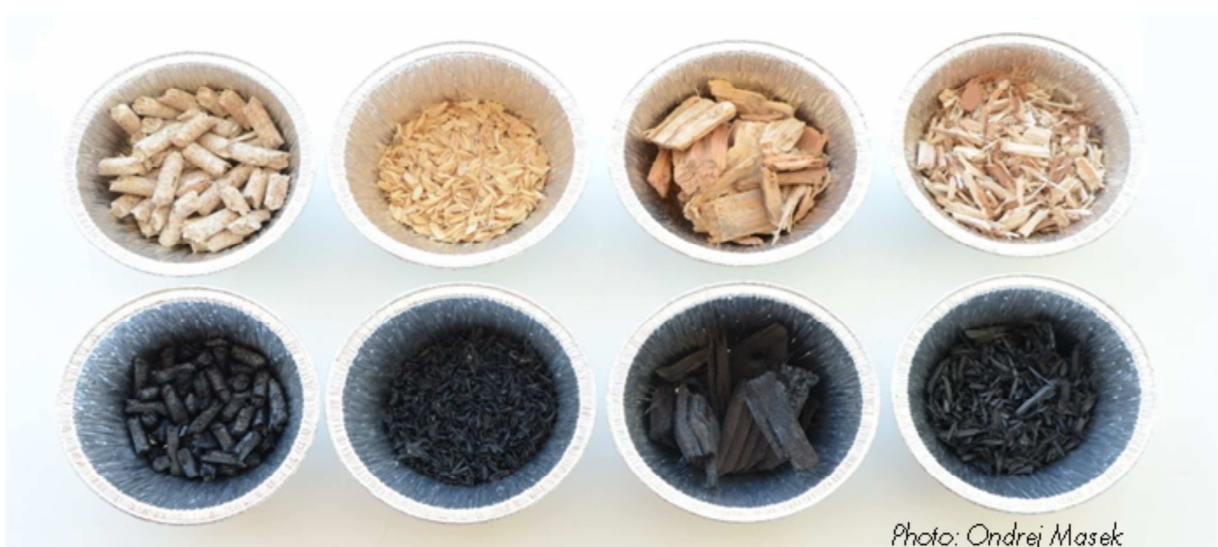
Figure 2.1: Biochar resembles the feedstock from which it is made; it can be made from a variety of materials such as – left to right – wood pellets, rice husk, wood chip, Miscanthus straw
