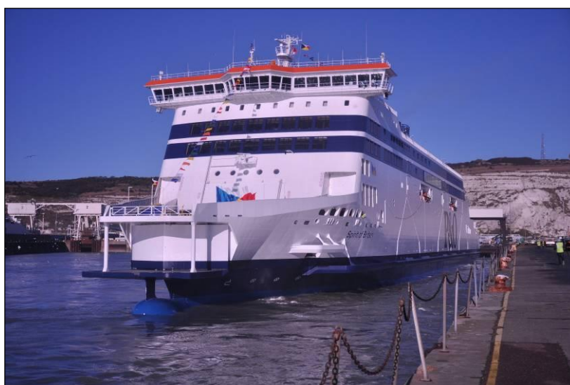
Image 3.2: Typical Dover type ferry with doors but no hinged doors / ramps
