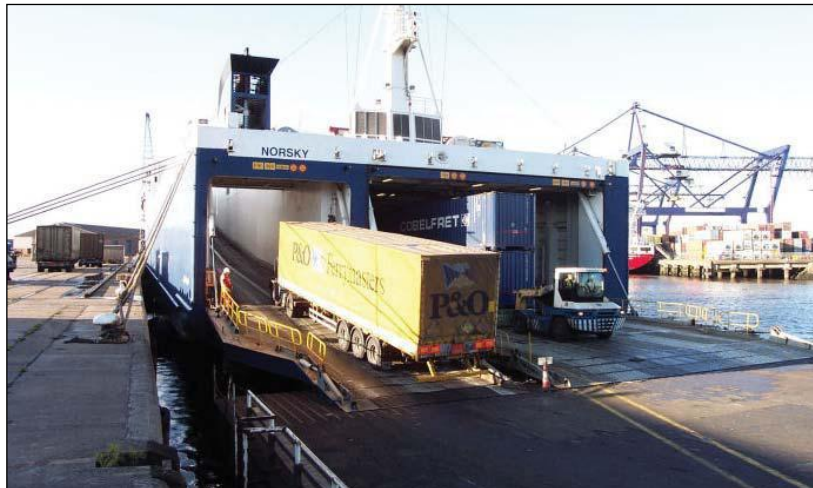
Image 6.2: RoRo vessel ramps / doors lowered onto the berth in port
