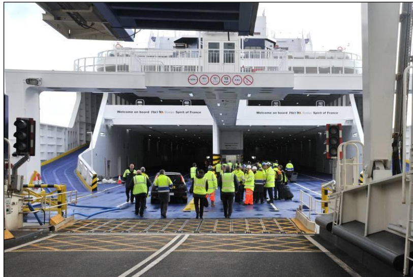
Image 6.1: Shore-side ramp lowered onto open deck of the Spirit of Britain in Dover (Dover type vessel)
